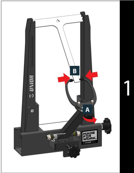
1689 professional wheel centering stand arm can get out of center after being used frequently. Controlling caliper arm enables us, to calibrate the stand arm back to its center position.
